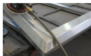
HANDWELDED CORNERS | Quality production produces durable canopies
